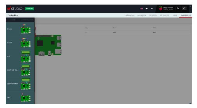
2. **The circuit image** It is located on the left side of the window. The image is interactive, meaning that the leds can turn on, the buttons can pe pressed, and so on.
