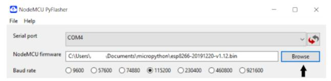
If you encounter errors, you need to reduce the baud rate (for example 9600 or up down). "1115200" is the speed read by serial port
